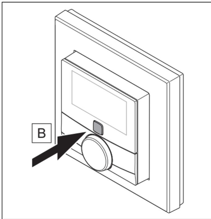
2. Re-insert the batteries in accordance with the polarity markings and, at the same time, press and hold the system button for four seconds until the signal LED starts to rapidly flash in orange.
