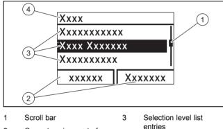
2 Current assignment of the and buttons. 4 Name of the selection level
