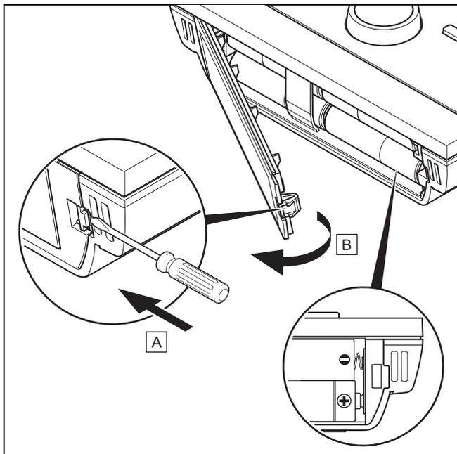
2. Insert four new batteries of the same type in the control.
