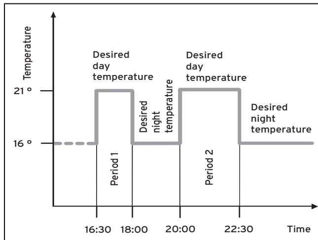
The **Time programmes** function can be used to set the time period for the heating circuit and hot water generation.
