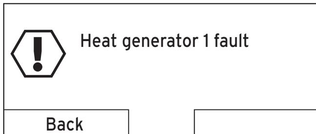
If the controller shows a fault message in the display instead of the basic display and you press the left-hand selection button **Back** then the basic display appears again.
