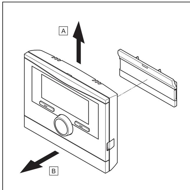
1. Remove the control as shown in the figure.
