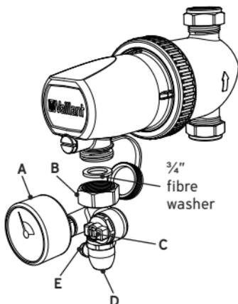
**A - Pressure Gauge:** The pressure Gauge is rated to Max 4Bar, if over pressure is encountered Drain point (E) can be opened to allow water safely out of the system via a hose, to a bucket or drain. This can be operated with a standard radiator bleed key.
