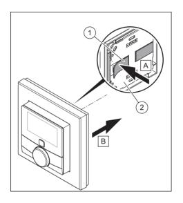
Secure the adhesive strips (1) to the rear of the mounting plate (2) in the markings provided for that purpose. Ensure that you can read the writing on
